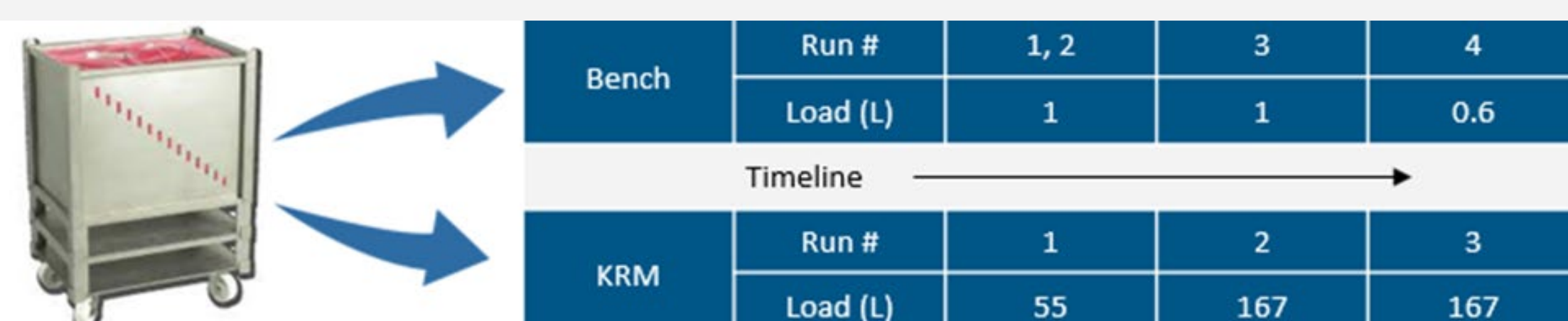
Figure 4. Experimental design for scale-up runs: one 55 and two 167 L, with their parallel bench-top runs.
